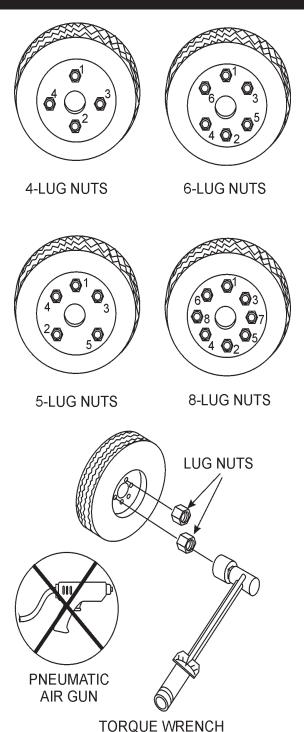
Figure 31. Wheel Lug Nuts Tightening Sequence
